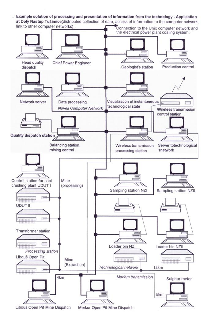
The information is processed and distributed by a computer network of the Novell type (network with ProfiBus communication protocol) 2 km long, the cable system is made up of classic telephone cables (RS485) laid along the mine.
